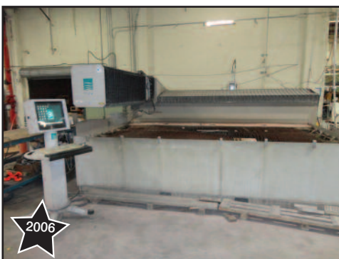
Flow Mod. 71633-1, 60,000psi Integrated Flying Bridge CNC Waterjet
