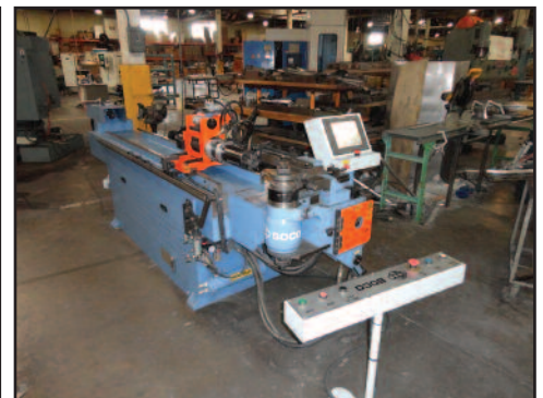
Soco Mod. SB-38NCMP, 1-3/8" Horiz. CNC Tube Bender
