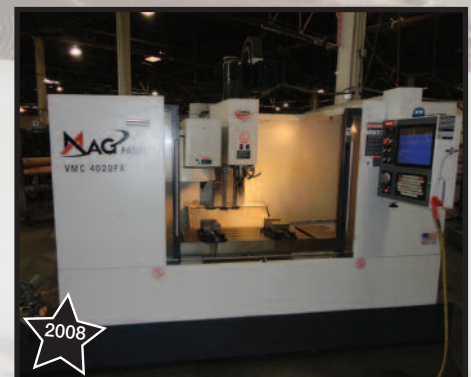
Fadal-Mag Mod. VMC4020FXMPHT Vert. Machine Center
