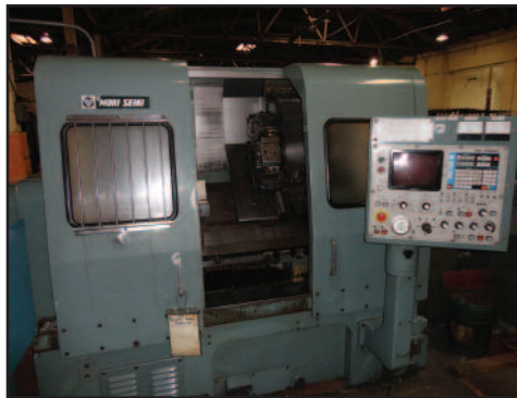
Mori Seiki Mod. SL3H CNC Turning Center
