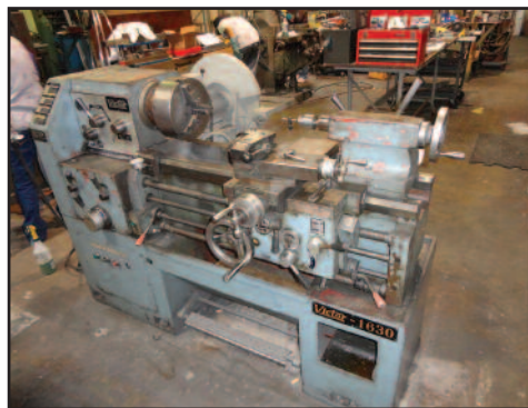
Victor 16"x30" Engine Lathe
