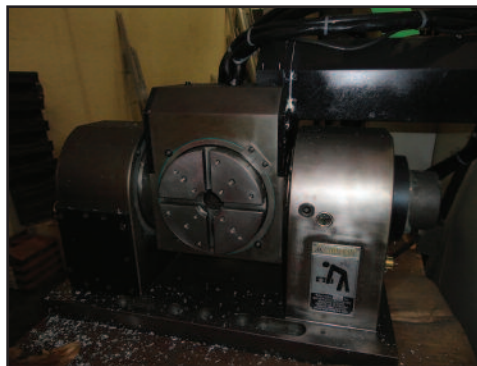
Fadal Mod. TR65 4th/5th Axis CNC Indexer
