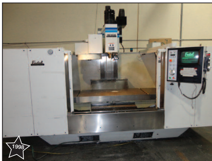
One of (2) Fadal Mod. VMC6030HT Vert. Machine Centers
