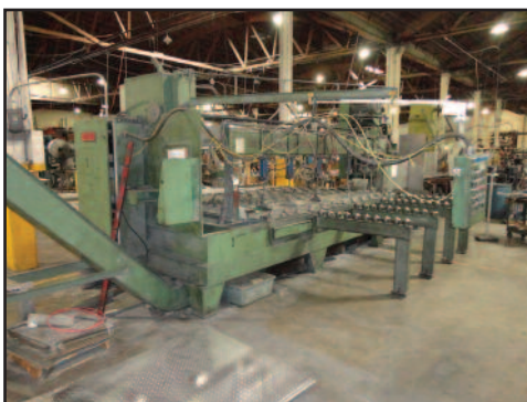
Savage 12' Alum. Plate Cross Cut Saw, 30hp
