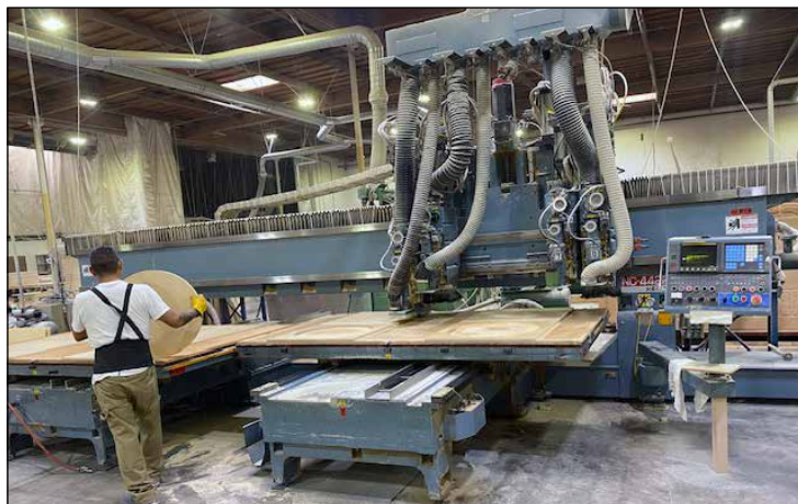
Heian NC-442P Vertical CNC Router
