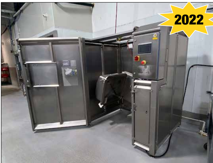
Syspal Type 600/SCM-1301, SWL 770lb. Bin Lifter
