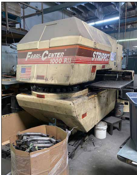
Strippit Fabri-Center 1000 RII CNC Turret Fabricator
