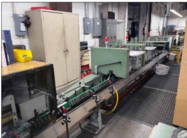
Mueller Martini Fold-Insert-Stitch Line
