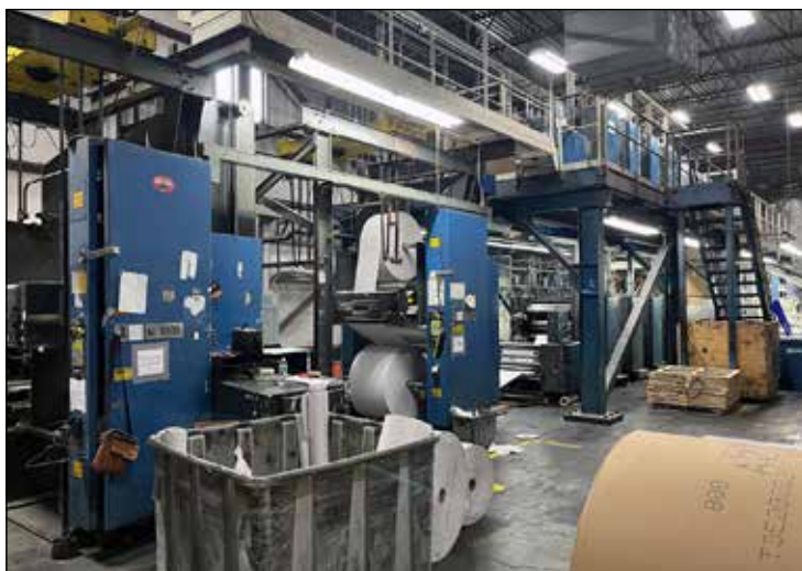
Harris V-30 Over-Under 4-Unit Press Line
