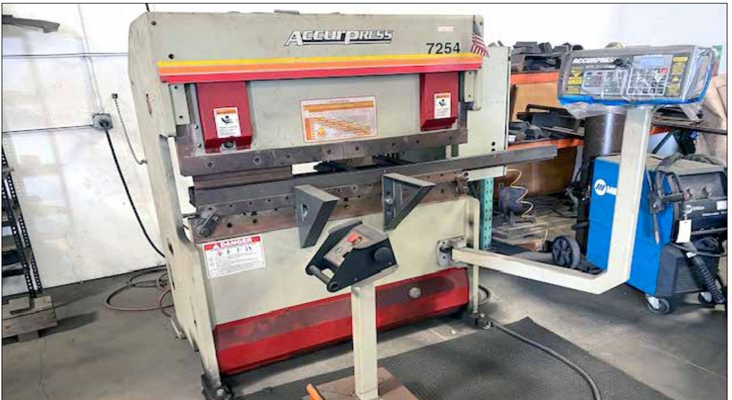
Accupress Mod. 7254, 6' x 25-Ton Power Press Brake
