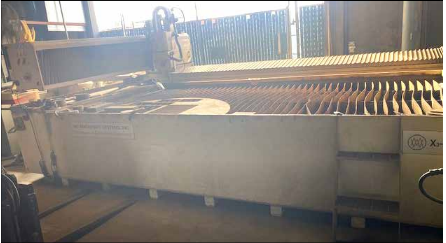
Mitsubishi MC Machinery Systems Mod. X3-612, Abrasive Water Jet
