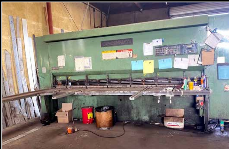
Cincinnati 500 x 12' Shear, 1/2" Capacity
