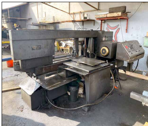
HEM Mod. Cyclone Auto-4, Horizontal Band Saw
