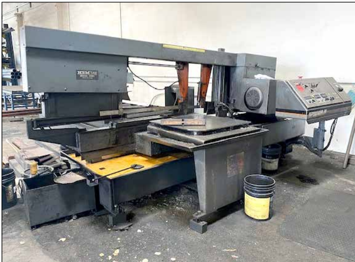
HEM Mod. SP2030HLM, Large Capacity Horizontal Band Saw
