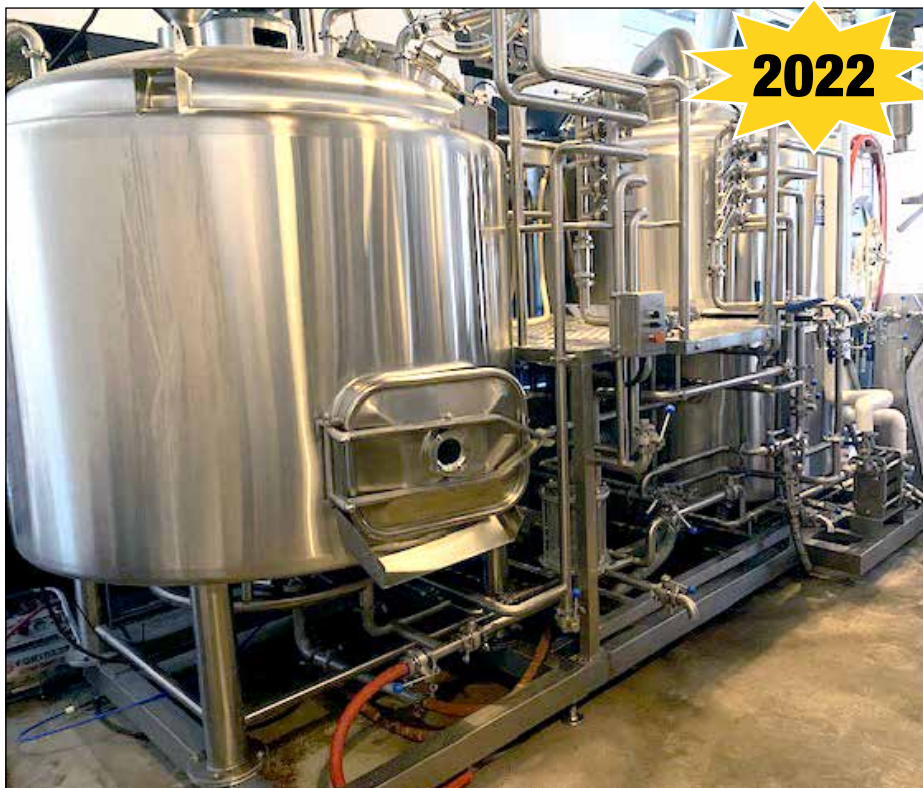
10BBL – 2 Vessel – Direct Fire Brewhouse, S.S. Brewhouse 304
