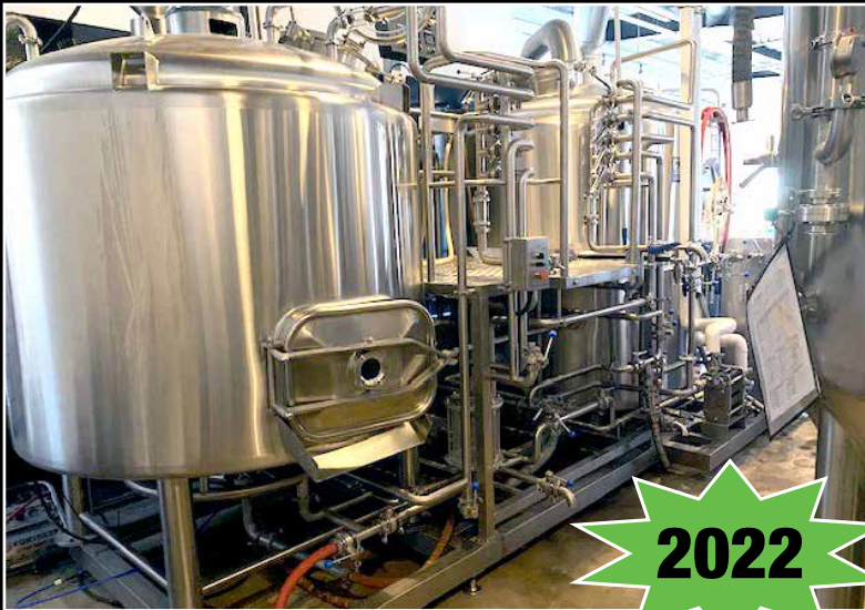
10BBL - 2 Vessel - Direct Fire Brewhouse, S.S. Brewhouse 304
