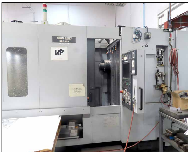
Mori Seiki Mod. NH5000, 4-Axis Horizontal Machine Center
