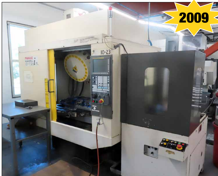
Fanuc Robodrill Mod. T21iFL, CNC Tapper
