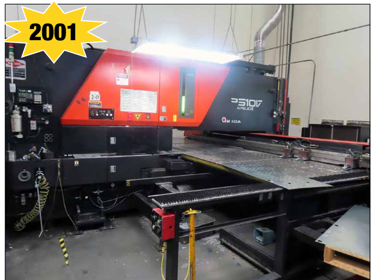
Amada Mod. Apelio 3/AP32510V, 5000 Watt CNC Laser/Turret Fabricator
