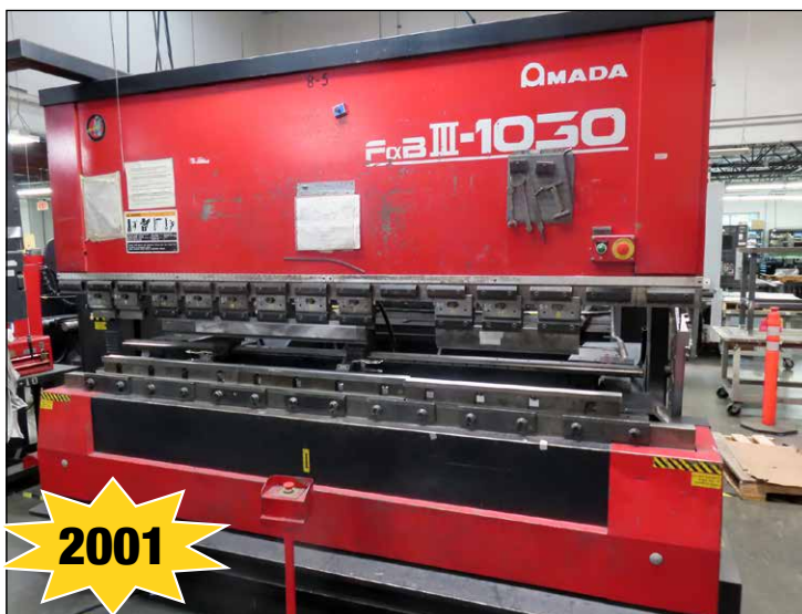
Amada FBD1030NT, 12' x 100-Ton CNC Press Brake
