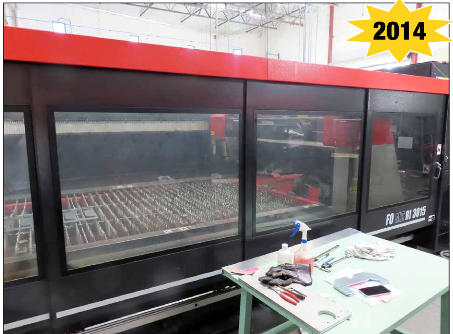
Amada Mod. FOM II R113015, 4000 Watt CNC Fiber Laser
