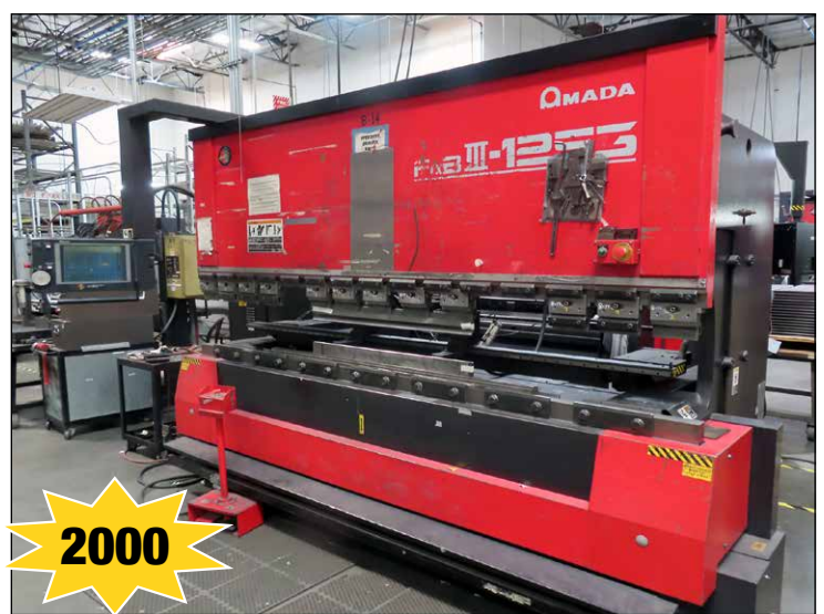
Amada Mod. FBD1253NT, 10' x 135-Ton CNC Press Brake
