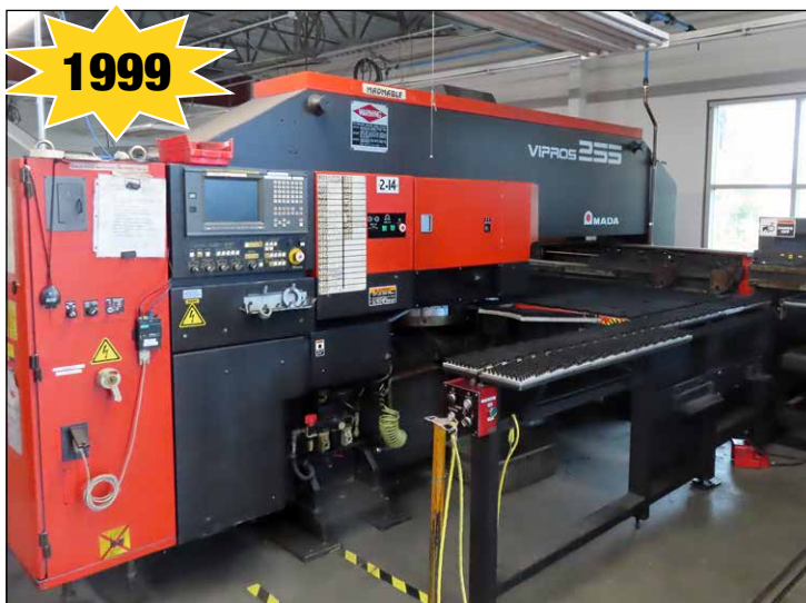
Amada Mod. Vipros 255, 22-Ton CNC Turret Fabricator
