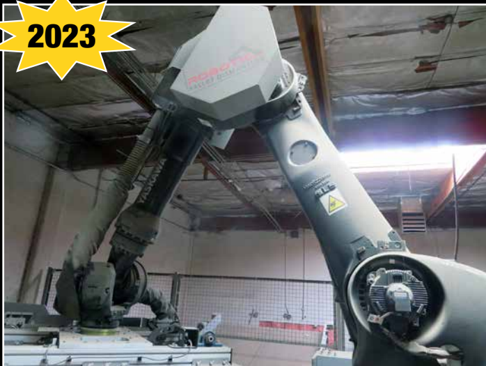
Alliance Robotic Pallet Dismantler w/Yaskawa Motomen HP3 Robotic Arm
