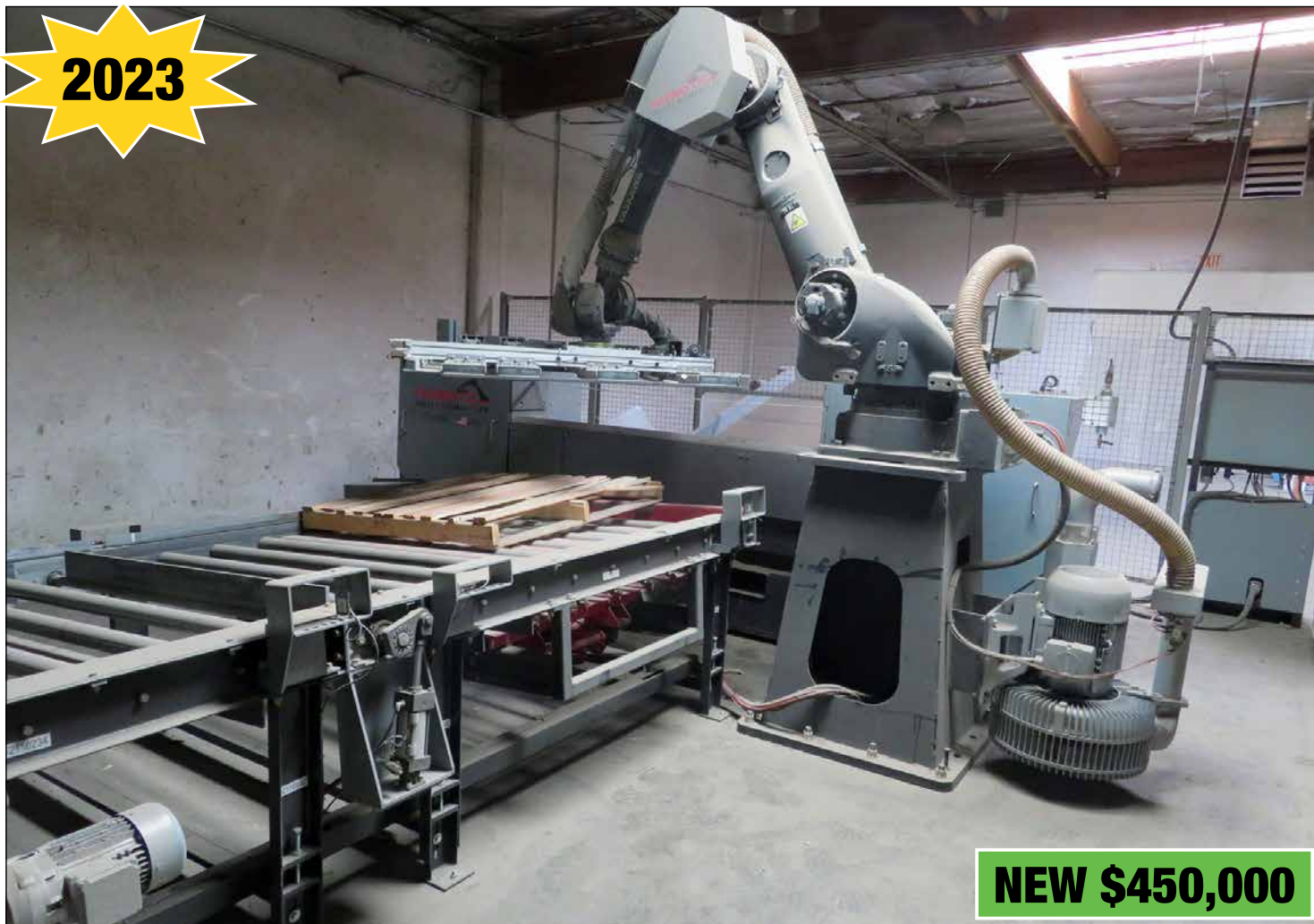
Alliance Robotic Pallet Dismantler w/Yaskawa Motomen HP3 Robotic Arm
