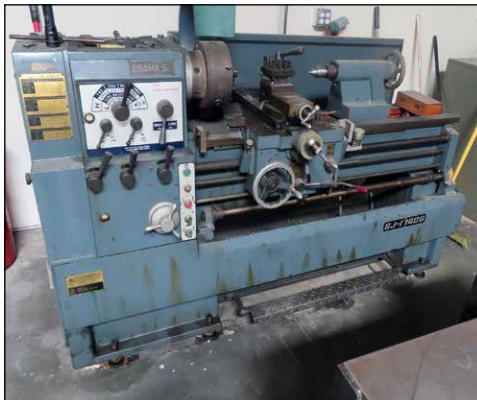
Osama Sr. SJ-1740G, 17" x 40" Gap Engine Lathe
