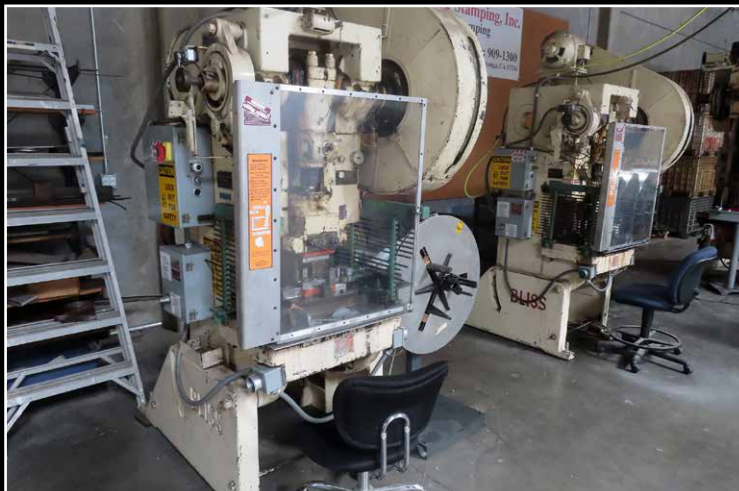
(2) Bliss Mod. C 35 Ton OBI Punch Presses
