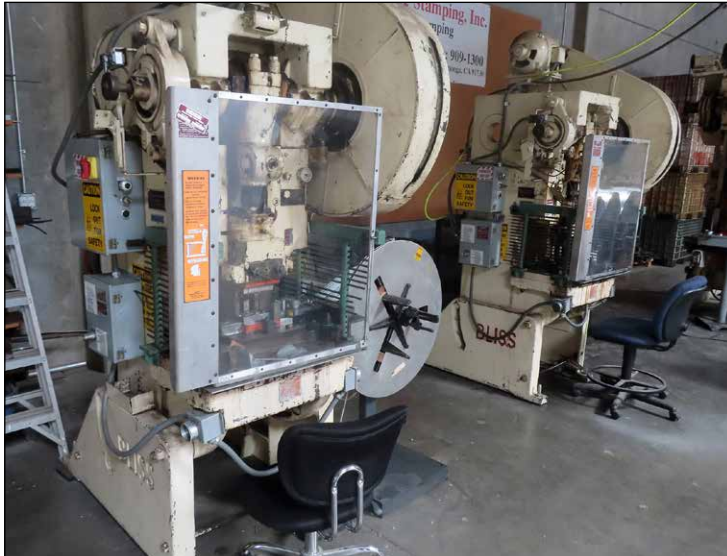
(2) Bliss Mod. C 35 Ton OBI Punch Presses
