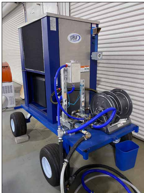
Cold Shot Mod. ACWC-036Q-LT06, Portable Chiller
