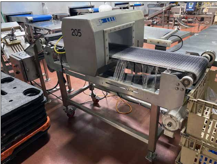
Loma Lock 30+, 8" x 4" Metal Detector and Bag Sealer
