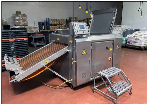
Ford Mod. CSPS-4C Counter Stacker
