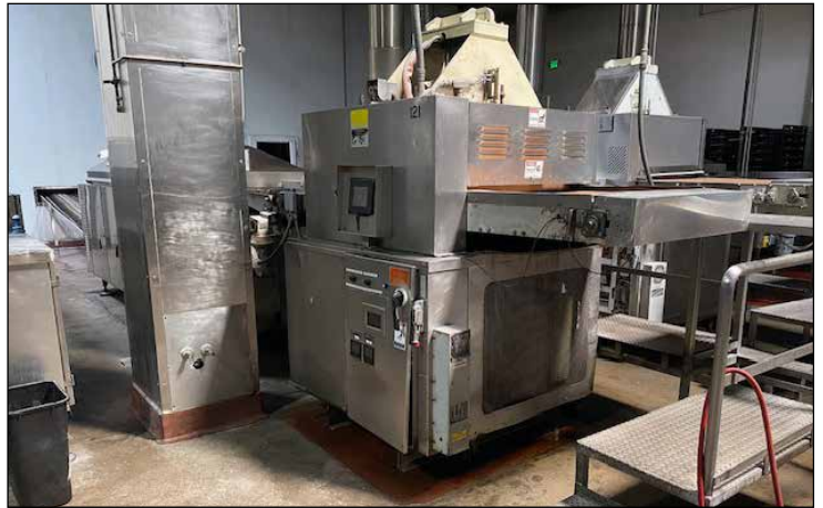
Casa Herrera Mod. HH1TP, 24" Conveyorized Tortilla Cooker
