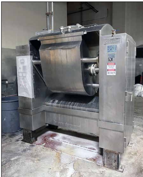
Peerless 300 Lb. Jacketed Roller Bar Dough Mixer
