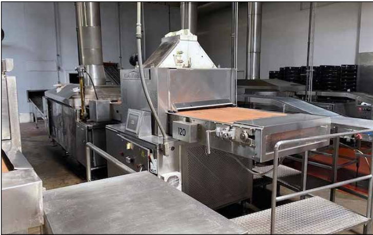
Casa Herrera Mod. TP3232, 32" Conveyorized Tortilla Cooker
