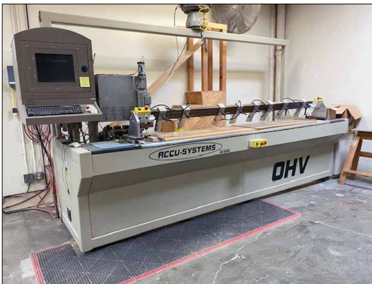
Accu-Systems OHV-ARCWOOD, Horizontal Fully Automatic Dowel & Drill Machine
