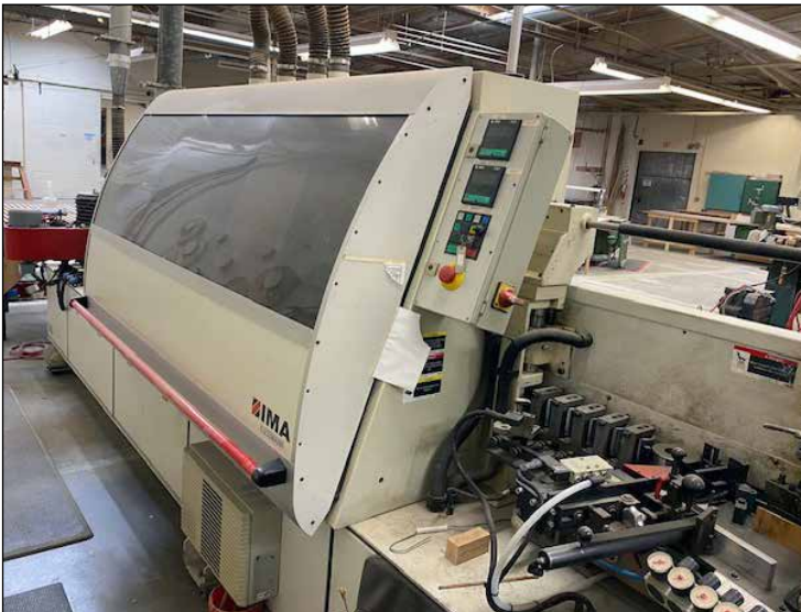
IMA Klessmann Type Advantage/5620/L Single Sided Fully Automated Edge Bander
