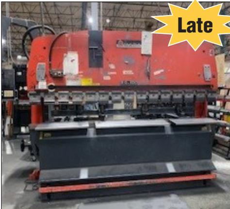
*Amada Mod. RG-100, 100-Ton Power Press Brake*
