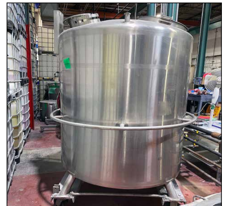
Will Flow S.S. Dimple Storage Tank
