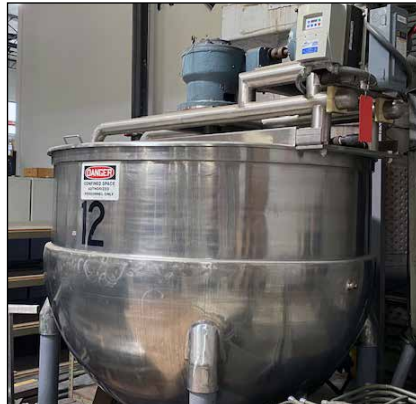
Crepaco 8,500 Kilo S.S. Tank, w/Sweep Agitation
