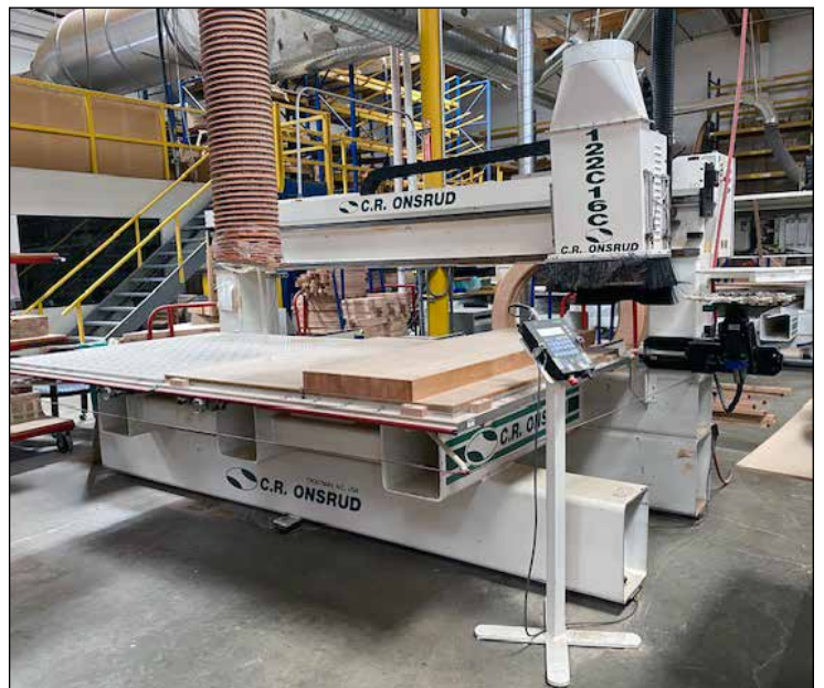
C.R. Onsrud Mod. 122C16C Vertical CNC Router
