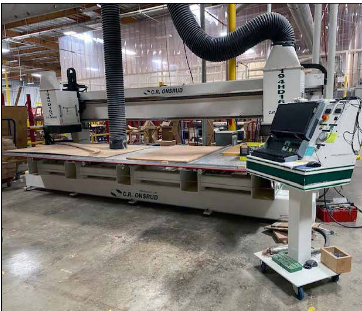
C.R. Onsrud Mod. 194HD16 Vertical CNC Router
