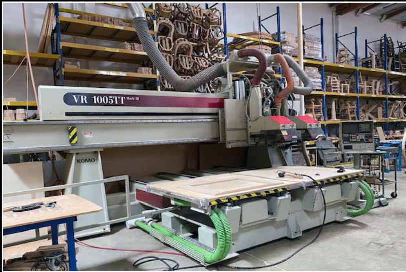
Komo Mod. VR 1005 TT Mach TTT Vertical CNC Router
