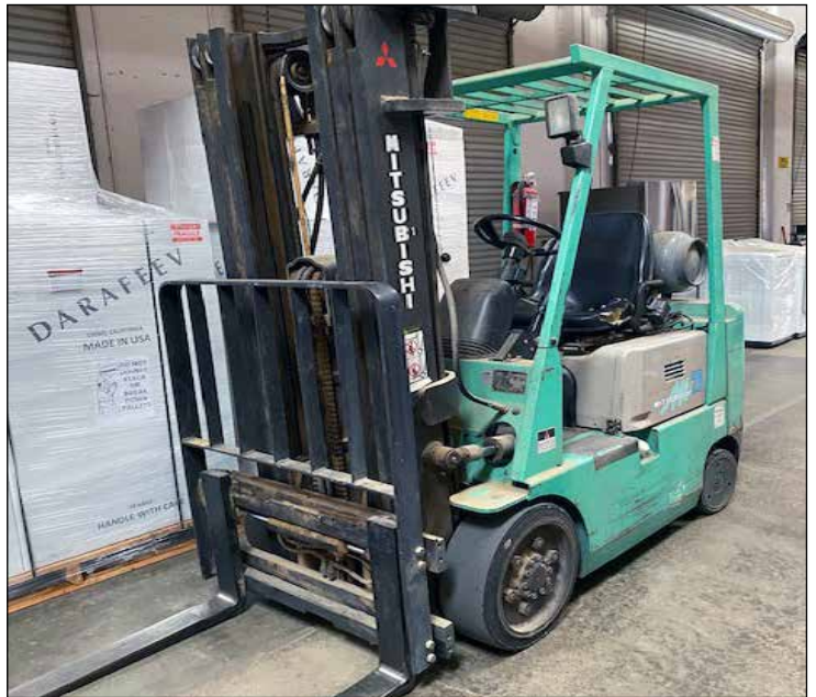
Mitsubishi FGC20, 4,000lb. LPG Forklift
