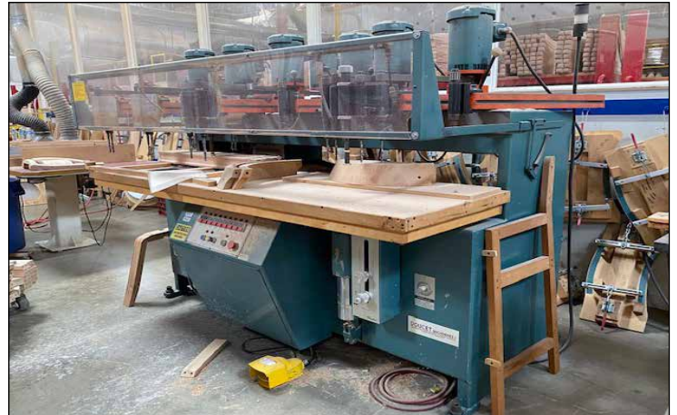
Doucet Mod. J3H-7 Multi Spindle Vertical Boring Machine
