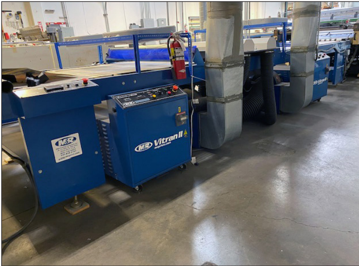
Vitson II, Mod VIT248202J, UV-Dryer Conveyor
