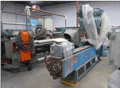
1974 Gloucester 3.5" Air Cooled Extruder
