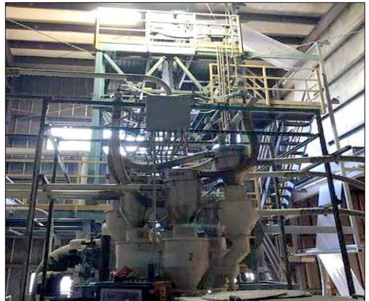
Brampton Engineering 4.5" Extruder with 250 Hp AC Drive
