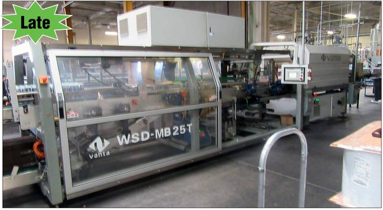
Venta Mod. WSD-MB 25T, Fully Automatic Shrink Film Wrapping Machine
