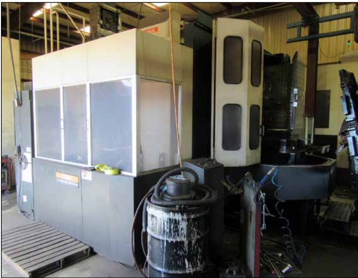
Mazak Mod. PMS, Pallettech High Rise System
