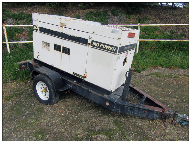
MQ Power Whisper Mod. DCA 25SS102 Watt 25KVA Diesel Powered AC Generator
