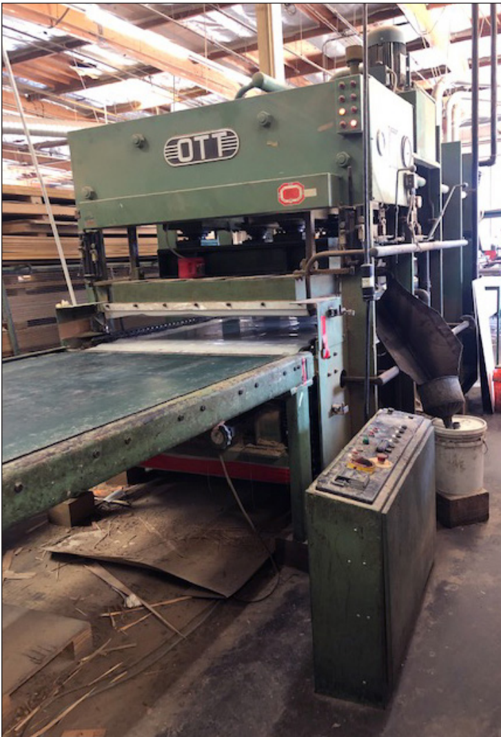
OTT Mod. D49-V/300, 56" Single Opening Hot Press
