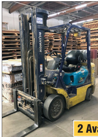
Komatsu 4,000lb. Capacity LPG Forklifts , w/Solid Tires and Overhead Guard
