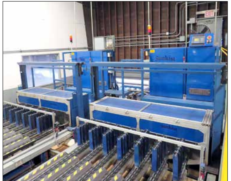
Partial View of Sunkist 14-Lane Color Sorter (Upgraded Software)
