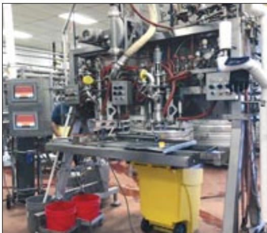
Aseptic Filling Line: Scholle Filler
