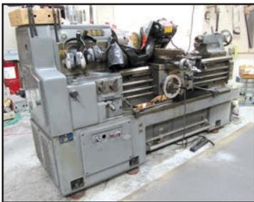
Webb 17"G x 40" Gap Bed Engine Lathe
