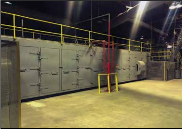
Views of Process Engineering 10' x 60' x 92" Conveyorized Curing Oven
