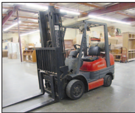
Toyota 5,000lb. LPG Forklift w/Side Shift
