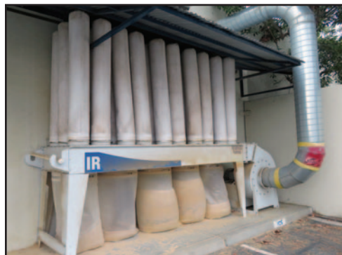
I.R. 25hp Dust Collection System w/Ducting
