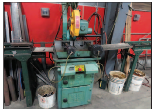
Doringer D350 Cold Saw w/Twin Clamping
