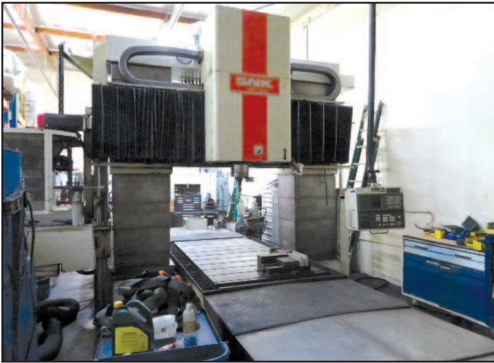
SNK RB2N Gantry Type Vertical Machining Center
