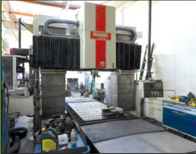
SNK RB2N Gantry Type Vertical Machining Center
