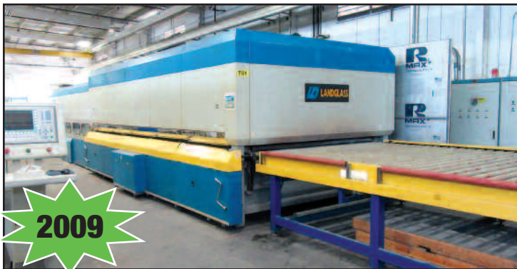
Landglass 8' Horizontal Roller Hearth Flat Bed Tempering Furnace
