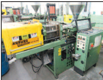
Arburg Injection Molder
