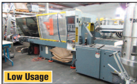
Engel Mod. ES1050/200TL, 200-Ton Injection Molder
