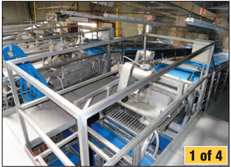
40" x 27' Sorting Belt w/Scalping Shakers
