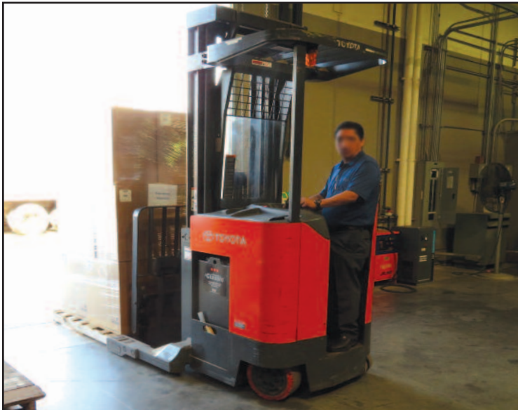
Toyota Mod. 7BRU18, 3500lb. Electric Stand-Up Forklift
