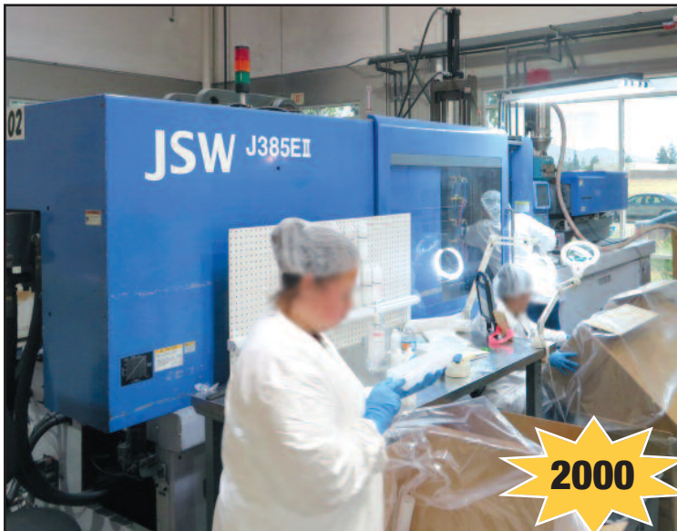
JSW Mod. J385EII, 385-Ton Injection Molder
