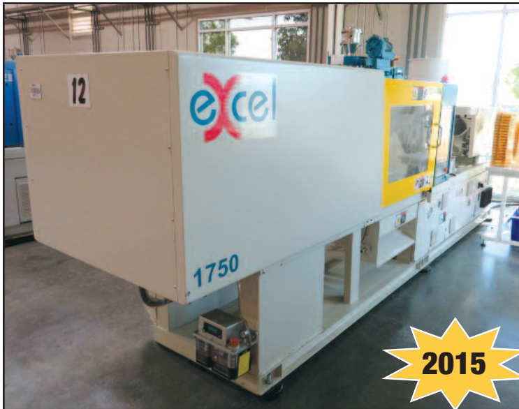
L.G. Excel Mod. PT160, 175-Ton Hybrid Electric/Hydraulic Injection Molder
