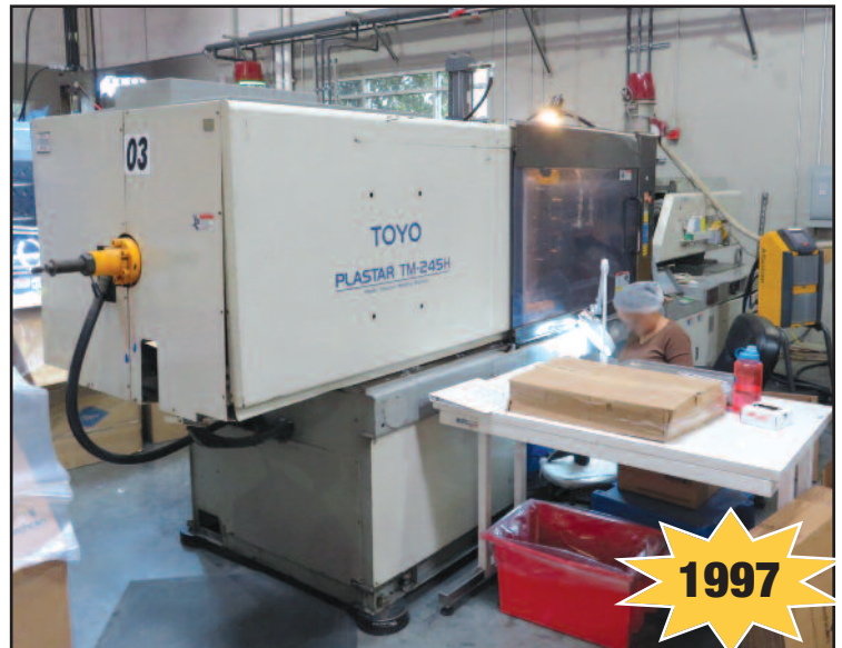
Toyo Plastar Mod. TM-245H, 245-Ton Injection Molder
