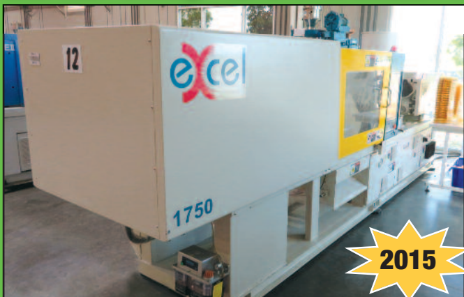
L.G. Excel Mod. PT160, 175-Ton Hybrid Electric/Hydraulic Injection Molder
