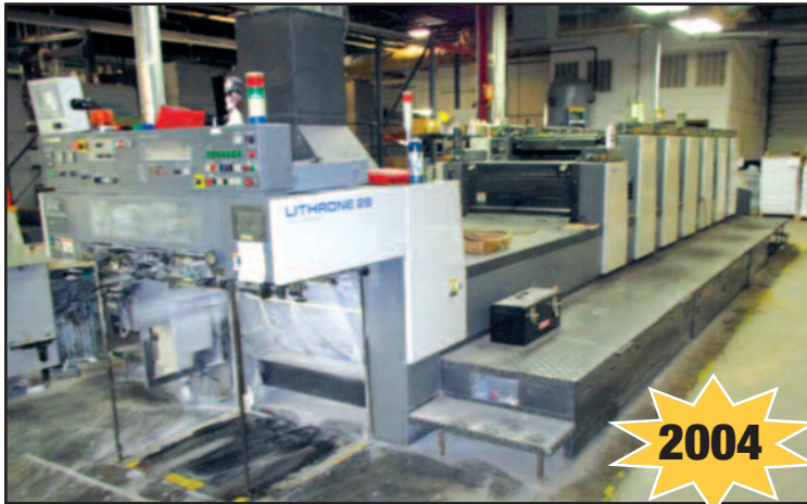
Komori Mod. Lithrone 28L-628, 20.47" x 28.47", 6-Color Sheet Fed Offset Printing Press
