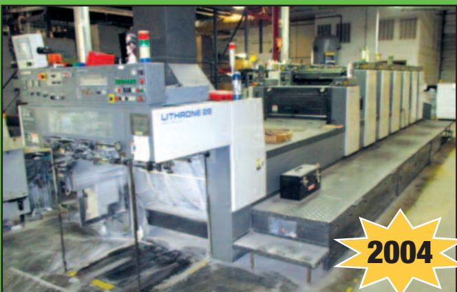
Komori Mod. Lithrone 28L-628, 6-Color Sheet Fed Offset Printing Press
