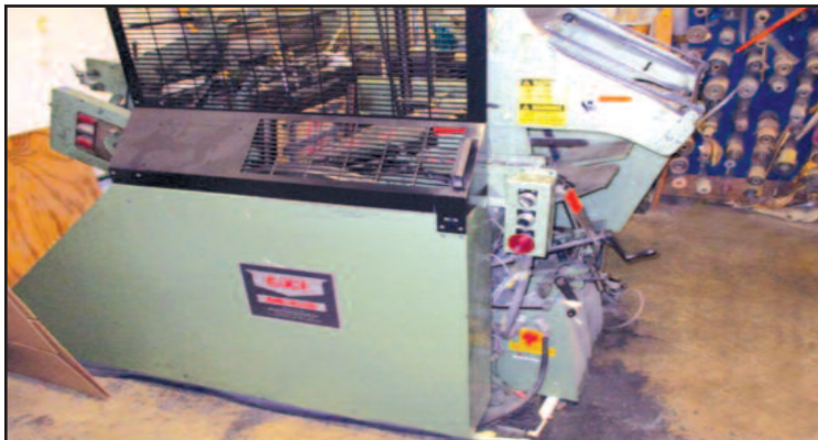
Kluge Mod. EHD, 14" x 22" Clam Shell Type Mech. Die Cutter
