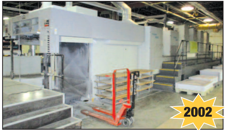
Man Roland Mod. R9046LV, 4-Color Large Format Carton Board Offset Printing Press
