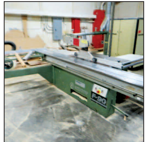
Altendorf Mod. F-90, 14" Sliding Table Saw
