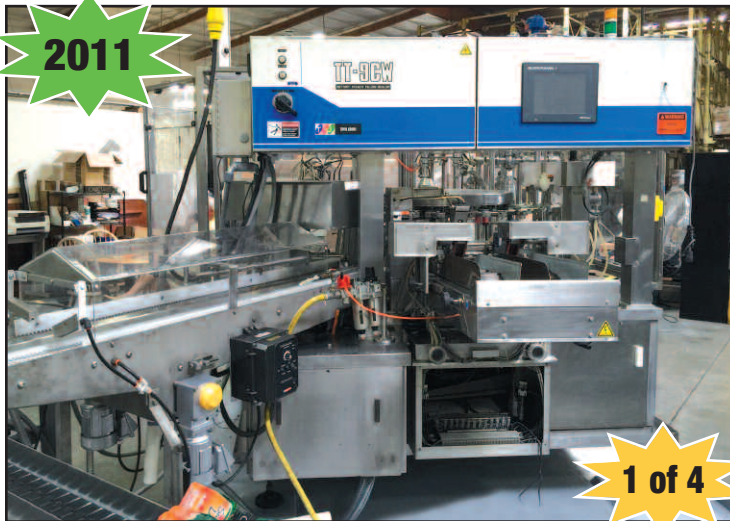
Toyo Jidoki mod. TT-9CW Auto. Rotary Retort Pouch Filler/Sealers
