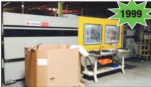
LG Goldstar mod. IDE 720EN Injection Molder
