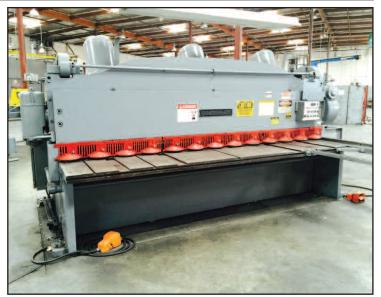
(1978) Cincinnati 2512, 12' x 3/8" Mild Steel Power Squaring Shear w/Front Operated Power Brake Gages, Front Extension & Squaring Arm, Maximum Capacity of: 0.375" x 12' Mild Steel, S/N 41757
