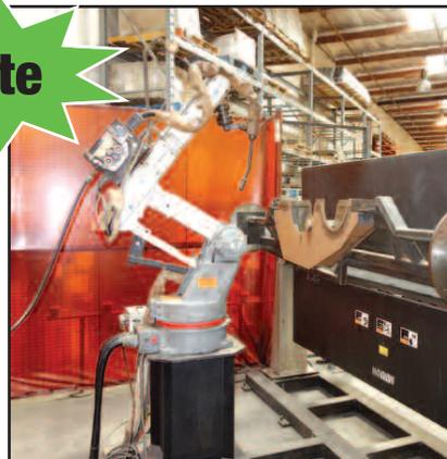
**Motoman Mod. Arc World 6000 K6SB 6-Axis Robotic Welder Including Seam Tracking and Torch Tender w/Motoman Yasnac ERC/K6SB Controls, Motoman/Hobart, RM2-150SB 7th Axis Positioner, Max Cap. of: 300lb x 39" Square x 102" Long. Hobart Mega-Mig Mod. RC-450 RVSS Power Supply S/N RPN 710-22314, 514068-1-2**
