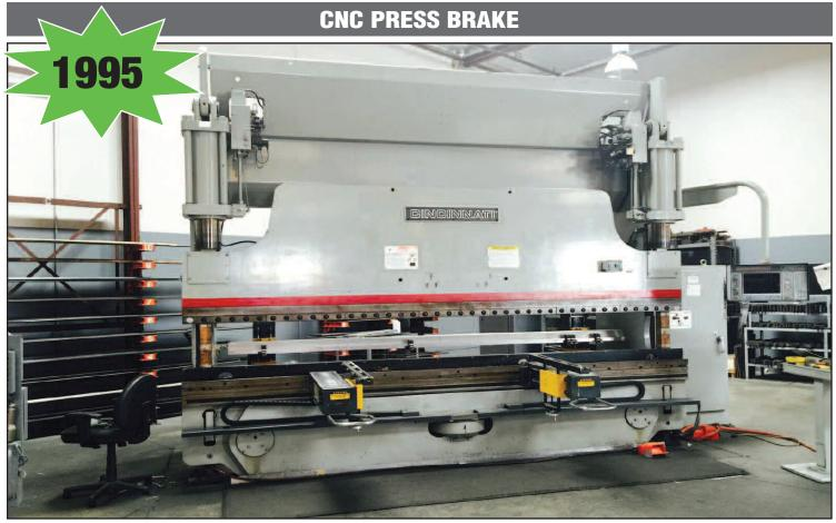
(1995) Cincinnati Autoform 175AF x 14ft. CNC Press Brake w/Cincinnati Adaptive Autoform CNC Controls Including CNC Front Gage, Custom 22" Max Stroke, 175 Ton Max Cap, Mild Steel Capacity is: 0.135" x 14', 0.188" x 12', 0.250" x 10', 0.375" x 6', S/N 48611
