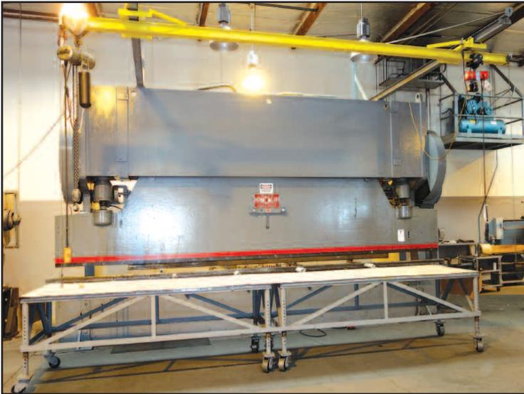
**Chicago Dreis & Krump Mod. 400-D-20, 24' x 266/400 Ton Power Press Brake, 24' Overall Bending Capacity; Mild Steel Capacity is: 0.188" x 24', 0.250" x 22', 0.313" x 7', 0.375" x 14', 0.500" x 13', 0.750" x 9', 1.00" x 6', S/N P9505**
