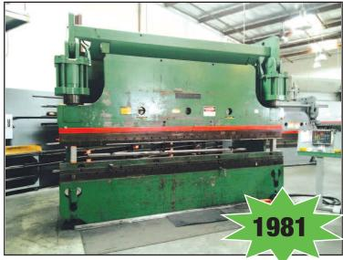
(1981) Cincinnati 350 CB x 14ft Programmable Power Press Brake w/Automec Controls, 10" Max Stroke, 350 Ton Max Capacity; Mild Steel Capacity is: 0.313" x 14', 0.375" x 12', 0.500" x 10', 0.750" x 8', 1.0" x 5', S/N 42272
