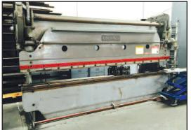
**Cincinnati** Mod. 1010, 10' x 135 Ton Power Press Brake w/14' Overall Bending Capacity, Maximum Capacity of 135 Tons; Mild Steel Cap. is: 0.120" x 14', 0.135" x 13', 0.188" x 10', 0.250" x 7', 0.375" x 4', 0.500" x 4', 0.750" x 3'
