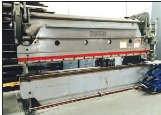
**Cincinnati Mod. 1010, 10' x 135 Ton Power Press Brake w/14' Overall Bending Capacity, Maximum Capacity of 135 Tons; Mild Steel Cap. is: 0.120" x 14', 0.135" x 13', 0.188" x 10', 0.250" x 7', 0.375" x 4', 0.500" x 4', 0.750" x 3'**
