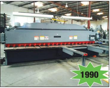
(1990) Cincinnati 2520, 20' x 10 Ga. Close Tolerance Mild Steel Power Squaring Shear w/Cincinnati Multi-Axis Gage Control Center, NC Front & Back Gages, (2) Front Extensions, Squaring Arm, Maximum Capacity of: 0.135" x 20' Mild Steel, S/N 46014
