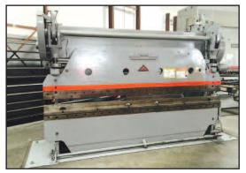
**Cincinnati** 5 Series 135 Ton x 12' Power Press Brake w/3" Stroke, Rated Cap.: at Midstroke 90 Ton, Near Bottom 135 Ton, Mild Steel Cap. is: 0.120" x 12', 0.135" x 12', 0.188" x 10', 0.250" x 7', 0.375" x 4', 0.500" x 4', 0.750" x 3', S/N 35081
