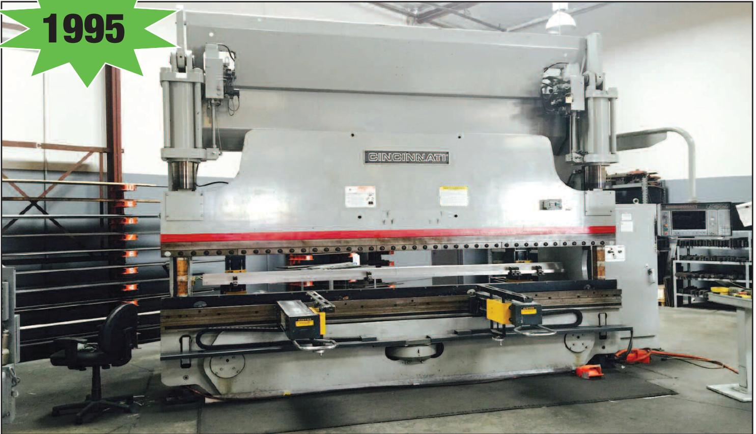
**(1995) Cincinnati Autoform 175AF x 14ft. CNC Press Brake w/Cincinnati Adaptive Autoform CNC Controls Including CNC Front Gage, Custom 22" Max Stroke, 175 Ton Max Cap, Mild Steel Capacity is: 0.135" x 14', 0.188" x 12', 0.250" x 10', 0.375" x 6', S/N 48611**
