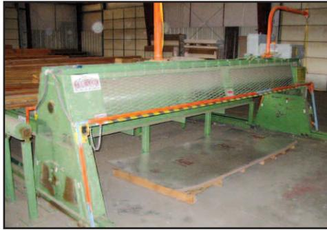
Tee Lok 14' x 24" Roller Type Gantry Truss Press
