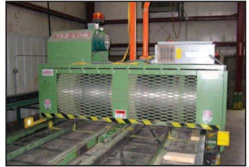
Tee Lok 6' x 24" Roller Type Gantry Truss Press
