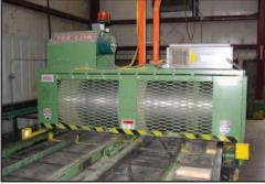
Tee Lok 6' x 24" Roller Type Gantry Truss Press
