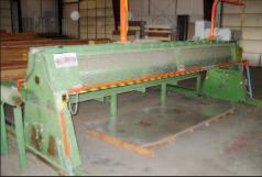
Tee Lok 14' x 24" Roller Type Gantry Truss Press
