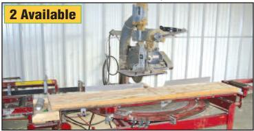
Speed Cut Mod. SSA17, Turntable Type Compound Saw
