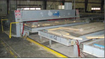
Klaisler G14-24, 14' x 24" Gantry Truss Press
