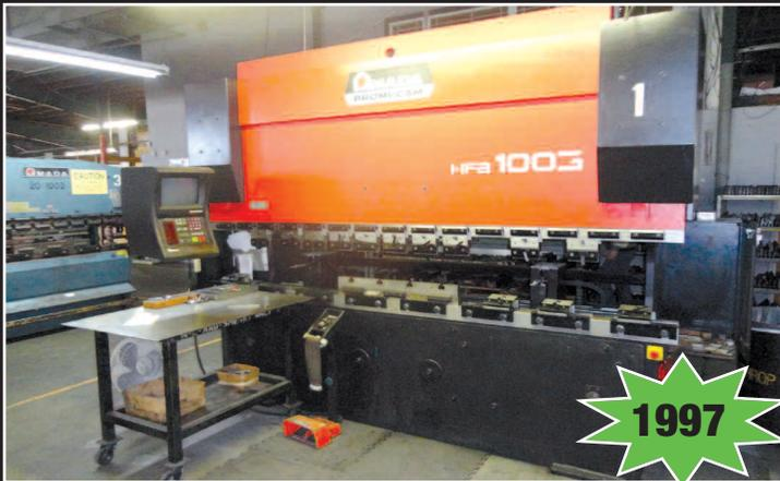
Amada Promecam HFB1003, 10'x110 Ton CNC Press Brake
