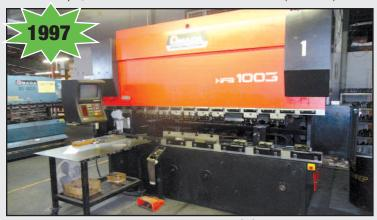
Amada Promecam HFB1003, 10'x110 Ton CNC Press Brake
