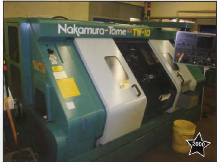
One of (2) Nakamura Tome Mod. TW-10, 5-Axis Dual-Spindle CNC Turning Centers
