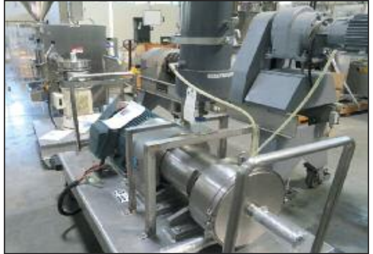
Ross 50hp Portable Homogenizer
