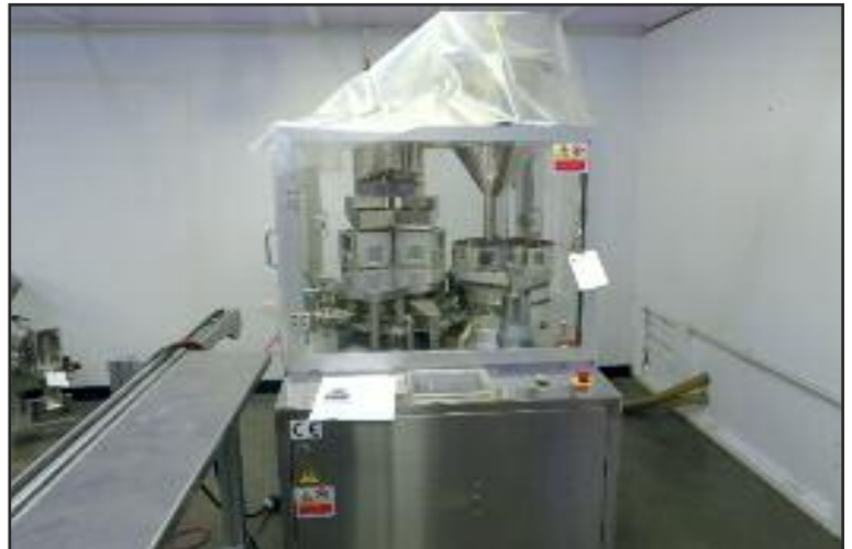
O & Size 1 Rotary Capsule Filler & Packager
