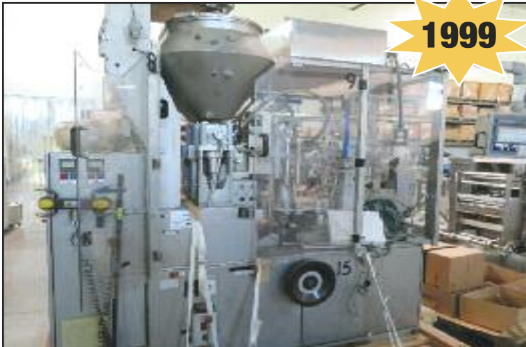
IWK Oyster Mod. TFS-30, 20-Station Tube Filler-Cassette Packager
