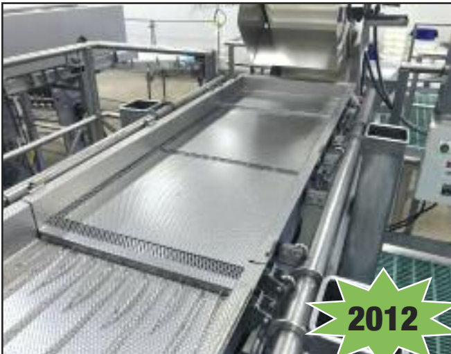
Meyer Vibratory Inspection Line
