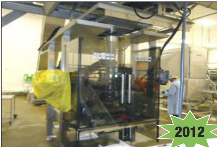
Matrix Triton Form-Fill-Bagger
