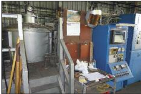
Wall Colmunoy Vacuum Furnace
