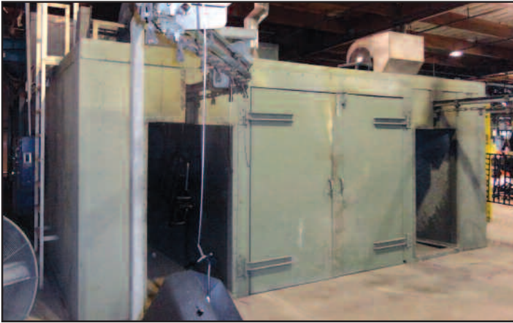
Views of Nordson Powder Coat Spray System
