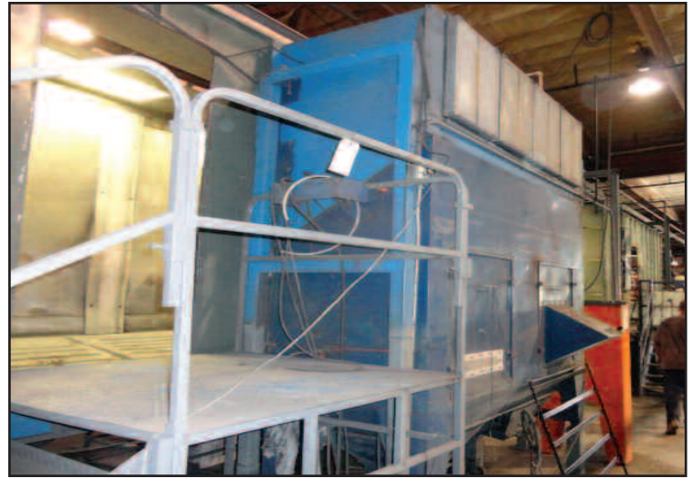
Views of Nordson Powder Coat Spray System
