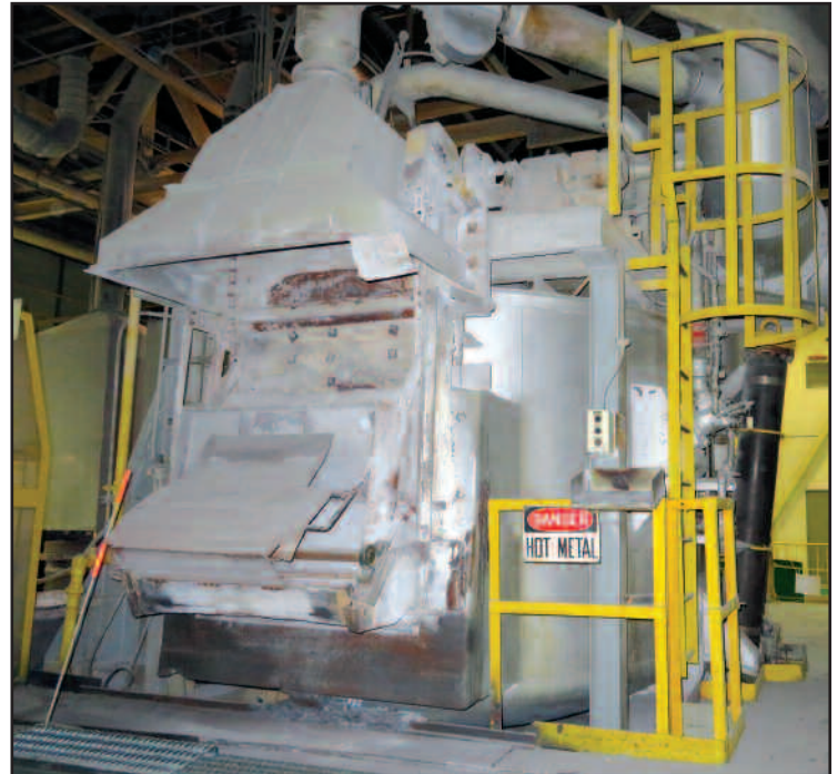
E&F Canefco 6,600lb. Alum Re-Melt Furnace
