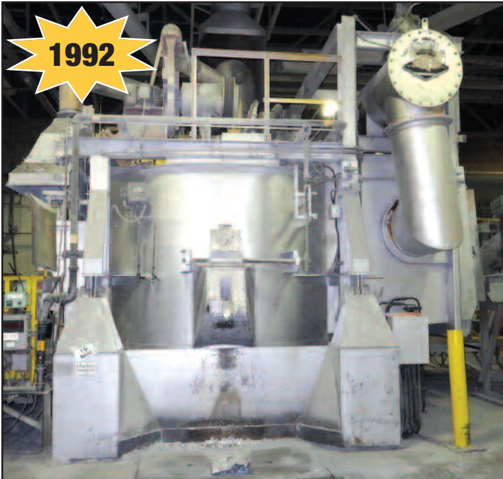
E&F Canefco 12,100lb. Alum. Re-Melt Furnace
