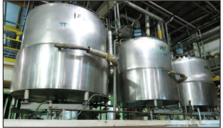
1750 Gal. Jacketed Sweep Agitated 316 S.S. Processing Tanks
