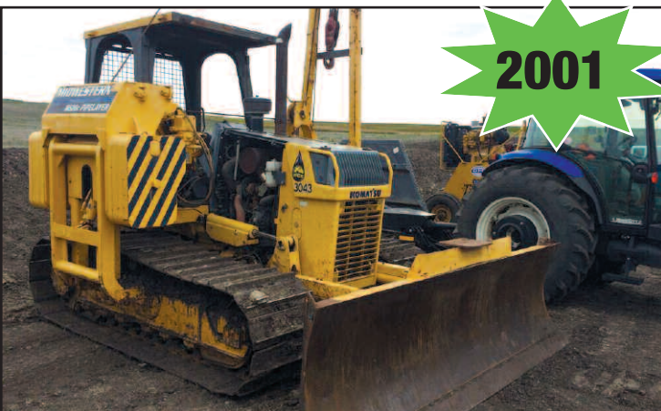
Komatsu D39PX Dozer w/ Pipe Layer Attachment
